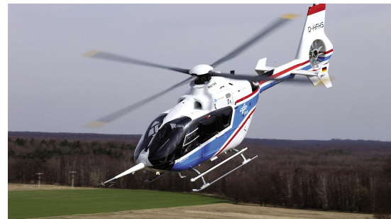
(b) DLR's ACT/FHS a heavily modified Eurocopter EC135, registration sign H-HFHS
