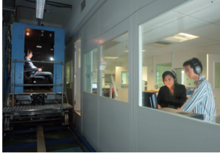
Figure 2.2: The 12m Tilting and Translating Cabin motion simulator of the Institute of Vibration at the University of Southampton. Taken from [36]
