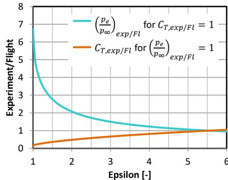
**Fig. 14: Exit pressure ratio similarity and thrust coefficient similarity as function of the nozzle expansion area ratio as in eq. (4) and (6) (for  $M_{\infty,Fl/exp}^2 = 1$ ). [15]**
