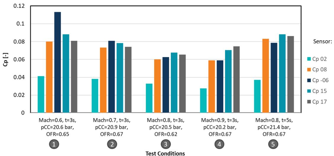
**Fig. 33: Pressure coefficients for the hot combustion tests**
