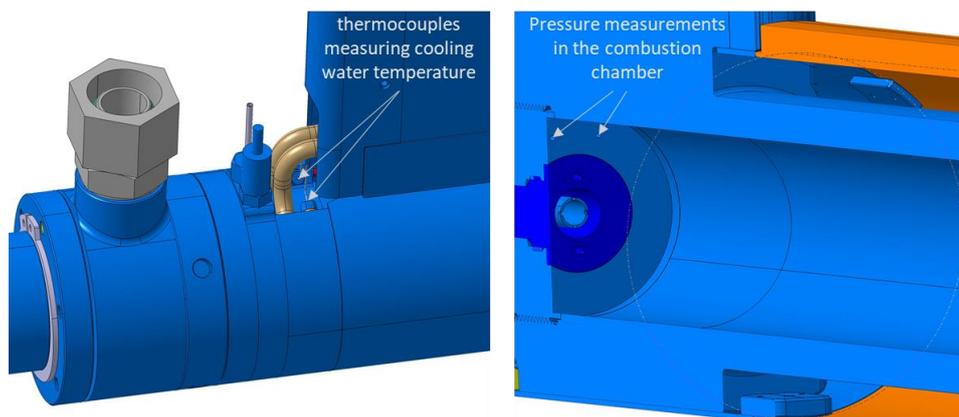
**Fig. 11: Temperature measurements of cooling water for the model's nozzle cooling (left) and pressure measurements in combustion chamber (right)**
