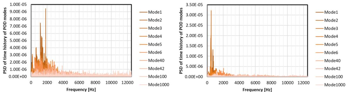
**Fig. 31: Power Spectral Density of time history of the POD modes (right singular vectors) of the cold gas case (left) and the hot gas case (right)**
