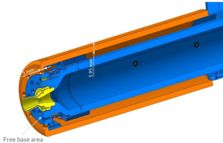
**Fig. 9. Outer cover for high heat loads**
