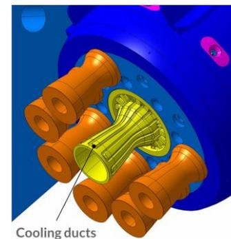
**Fig. 8: Central nozzle with transparent view on cooling ducts**
