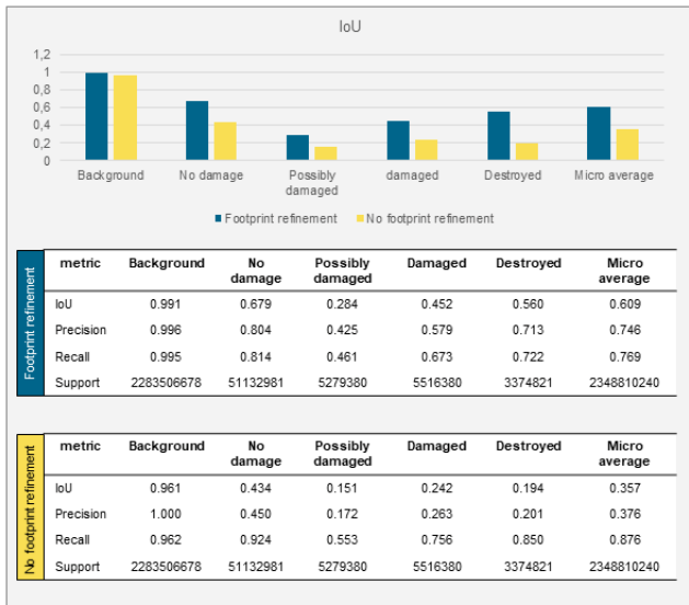
Figure 2: Accuracy assessment of the Siamese U-Net model with and without building footprint refinement on an independent test split of the xBD dataset.
