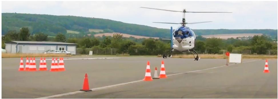
**Fig. 2** CoAX2D during acceleration/deceleration MTE evaluation [2]. Cones and ground markings are used as visual cues
