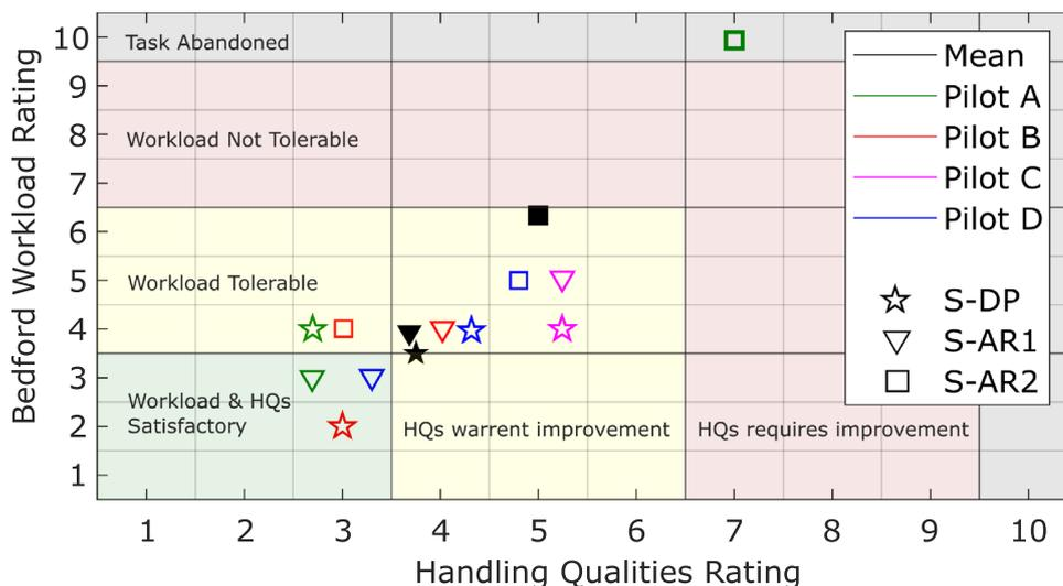
**Fig. 12** Bedford Workload Ratings and Cooper–Harper Ratings for MTE Slalom
