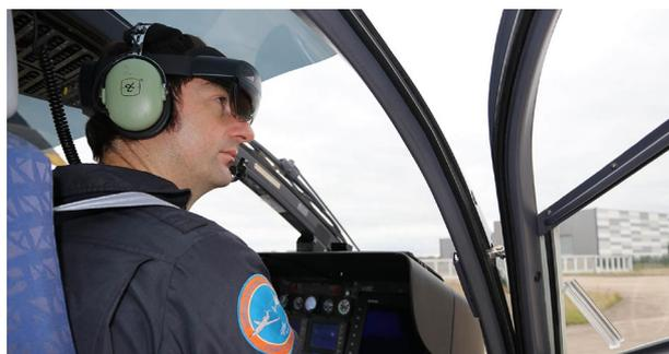
Fig. 3 Microsoft HoloLens 2 as HMD in DLRs ACT/FHS cockpit
