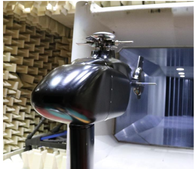
Figure 22: REF fuselage with dummy rotor system at DNW-NWB
