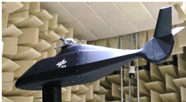
Figure 11: 3D-printed REF fuselage (top), SZ-1 fuselage (bottom)
