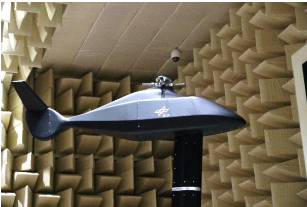
Figure 24: SZ-1 fuselage with dummy rotor system at DNW-NWB
