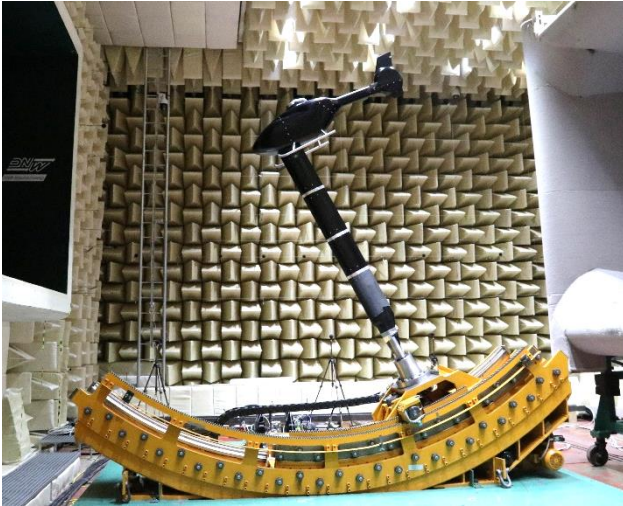
Figure 23: REF fuselage with skids without rotor
