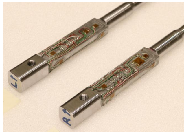
Figure 13: Wing balance strain gauge instrumentation
