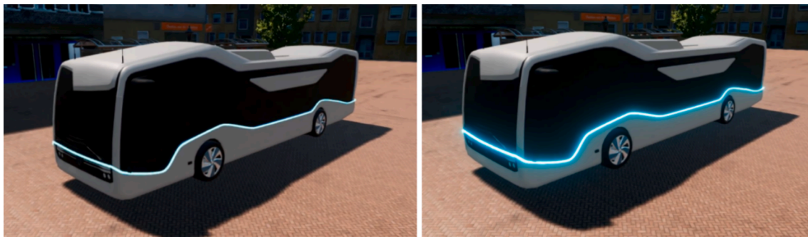
Fig. 3. Demonstration of the static eHMI (left) and pulsation of the dynamic eHMI (right) for the bus.
