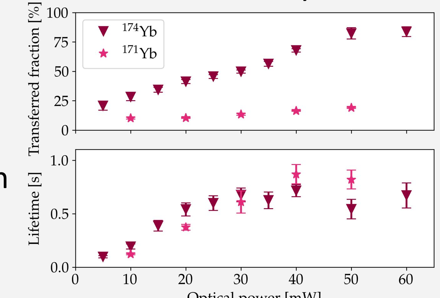
First demonstration of 2<sup>nd</sup> stage cooling of a fermionic alkaline-earth-like isotope in a non-conventional MOT geometry!
