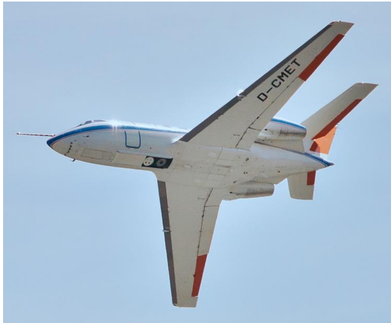
Figure 1. DLR research aircraft Dassault Falcon 20 (D-CMET) with opened bottom flap showing circular windows for LDA and FRS (rearward, grey/black). Image copyright: DLR / Kliebisch.
