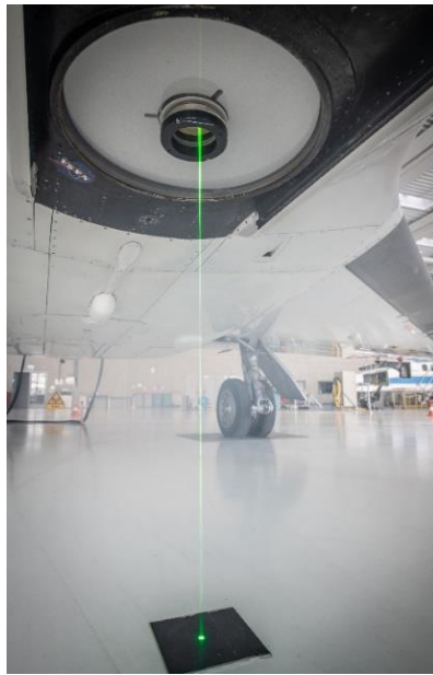
Figure 5. FRS laser beam during ground adjustment, the central part of a larger LIDAR window is used (outer area shielded). Image copyright: DLR / Riedel.
