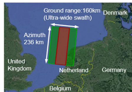
Fig. 2 North Sea test site selected for the experimental acquisition. The green rectangle delimits the 160-km ground swath area of the acquired SAR image, while the red rectangle delimits the area within the 66-km ground swath from the 3-dB antenna beamwidth.
