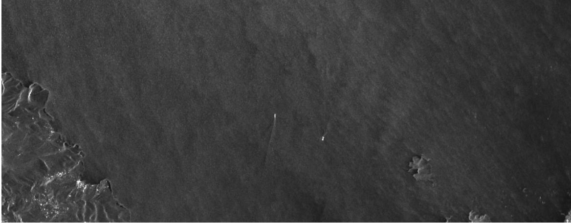
Figure 1. TerraSAR-X image acquired over the Saronic Gulf focused on MPSoC including coastal areas and bright scatterers on sea. The scene covers 33.5 km in range and 13.1 km in azimuth direction. TerraSAR-X data © DLR 2016.
