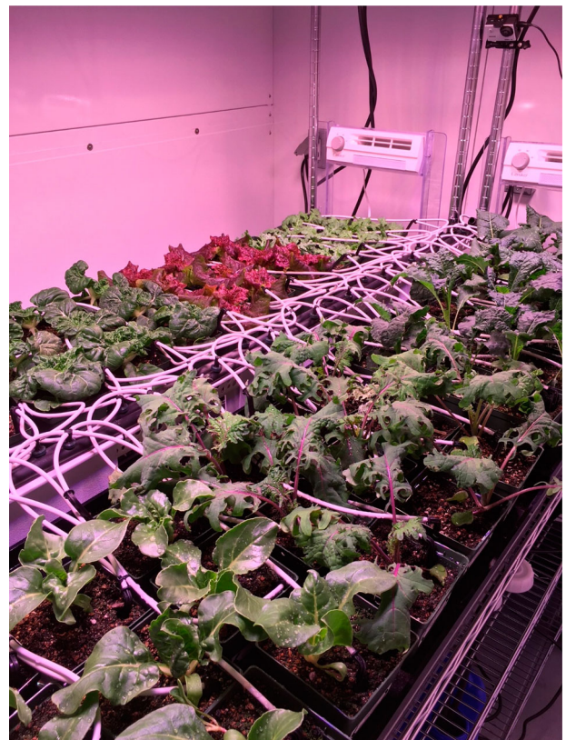
Figure 1. Leafy vegetable crops grown in a controlled environment chamber to study CO_2 effects. White tubes are irrigation drip lines. All plants were grown in 10-cm square pots and watered to excess several times daily with a complete nutrient solution.
