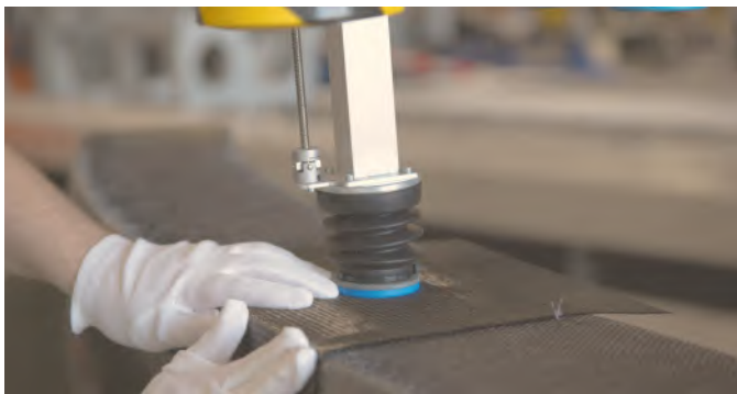
Fig. 7. Draping of small patch. One suction unit is holding the material firm on the mould, while the human can use both hands for precise draping.
