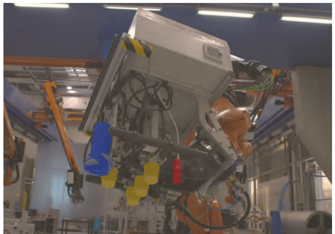
Fig. 6. One of the grippers provided by Abele Ingenieure GmbH. You can see the four suction units (yellow), the fibre angle sensor (blue) and the camera for “take picture” action (red)
