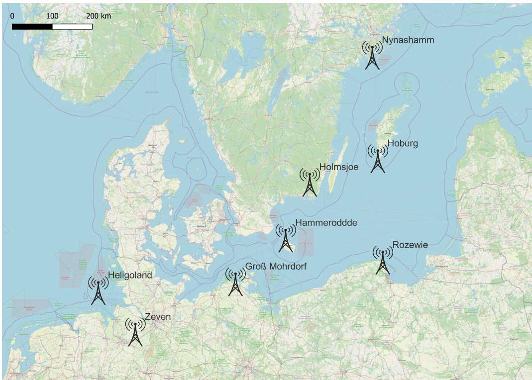
Figure 1.1: Testbed R-Mode Baltic: MF station operated in February 2021.
