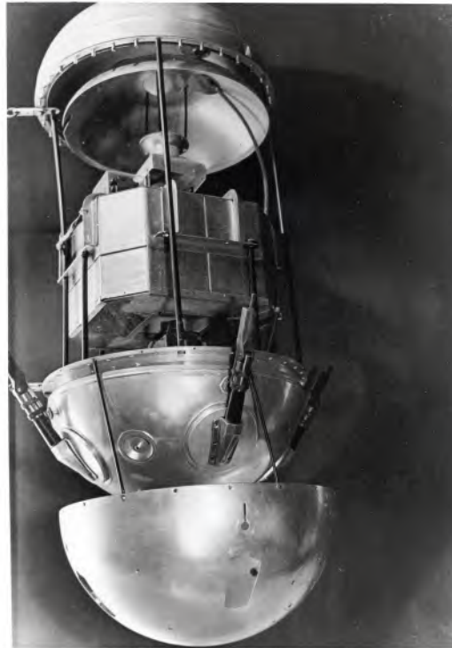
(b) Detailed exploded view of Sputnik 1, illustrating its internal components and construction.
