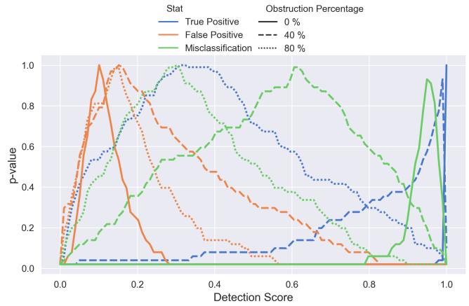
KS Test p-value as Function of the Detection Score for Law Enforcement Ships
