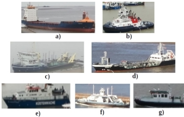
Fig. 1. Examples extracted from ShipSG that show the seven ship classes. (a) Cargo, (b) Tug, (c) Special 1, (d) Tanker, (e) Law Enforcement, (f) Passenger/Pleasure, (g) Special 2
