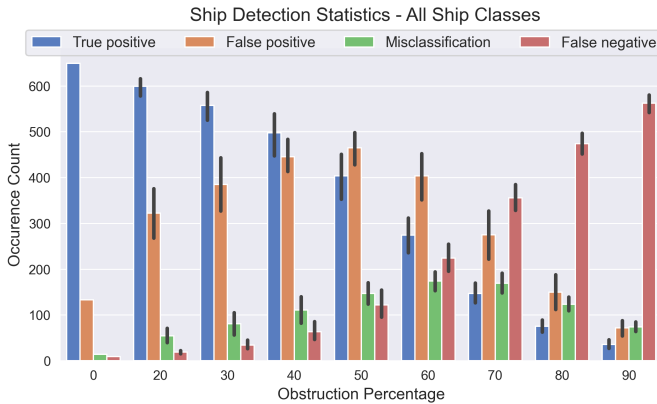
Fig. 3. Relationship between the occurrence of the evaluated stats of interest and the obstruction rate, given as a percentage of the ship bounding box being occluded.
