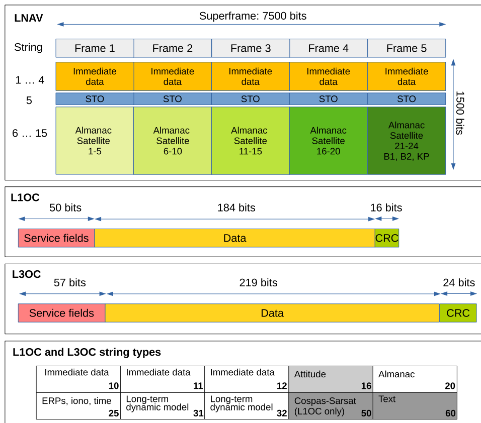
Fig. 2. Structure of GLONASS FDMA and CDMA navigation messages. CRC: cyclic redundancy check; STO: system time offsets. B1 and B2 describe the difference between UT1 and UTC(SU). KP is a leap second flag. String types shaded in gray are transmitted only on a per-needed basis, while white indicates strings that are currently transmitted at regular intervals.
