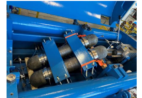
Single-tube-prototype in cyclic pressure test
