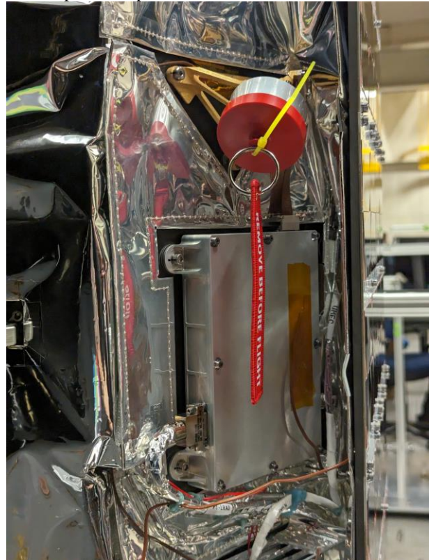
Fig. 1: LRAD instrument with sensor head on PEEK bracket and avionics box integrated into the S.P.Hopper behind the solar panel
