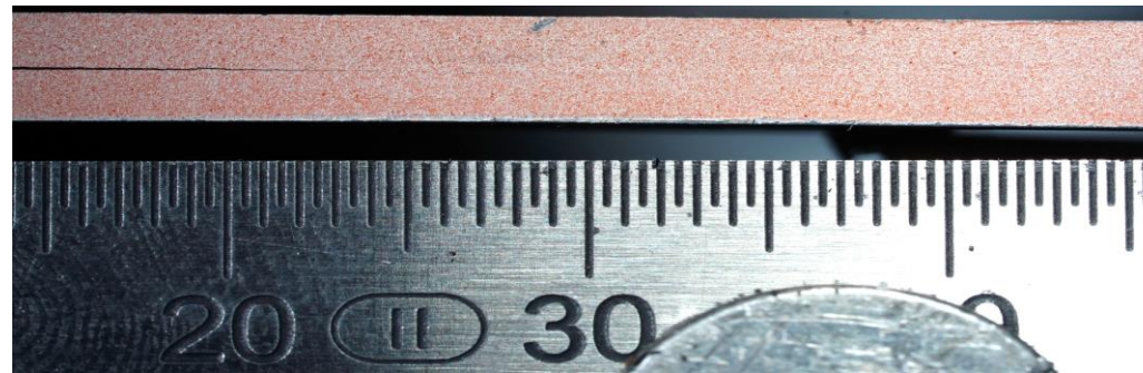
Crack detection of CLS specimen ST_01 3000\mu\text{m m}^{-1} at 1\text{M} cycles
