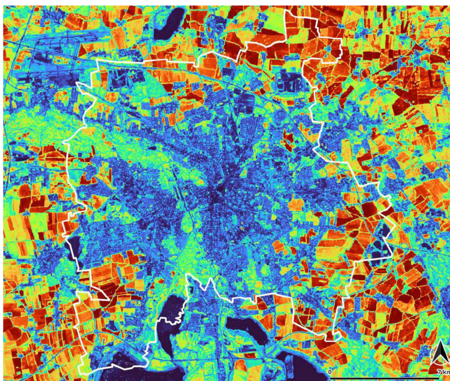
Figure 4. The indicator Variance is calculated separately for each channel. In the result, each channel gives the median of a Landsat 8/9 time series from 2018–2023. The square of the standard deviation is the variance. In this case, the time variance reaches 0.02 or 45% deviation from the mean of the NirV index. Landsat 8/9 time series, May to October from 2018 to 2023, Leipzig region, Germany.
