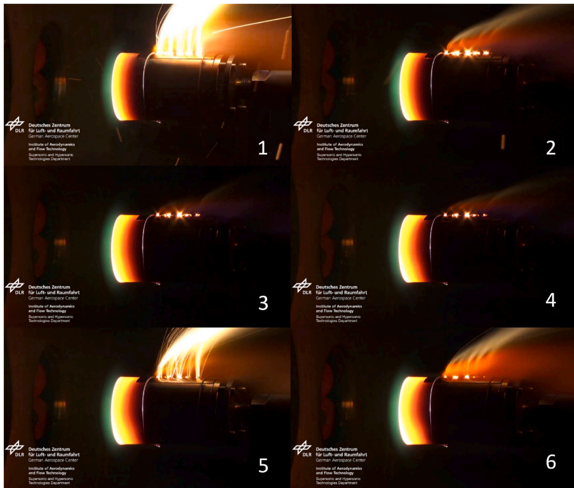
Fig. 11. Unsteady ejection from thin-walled BBU geometry, Test 12. Each frame is captured with a time interval of 0.2 s.
