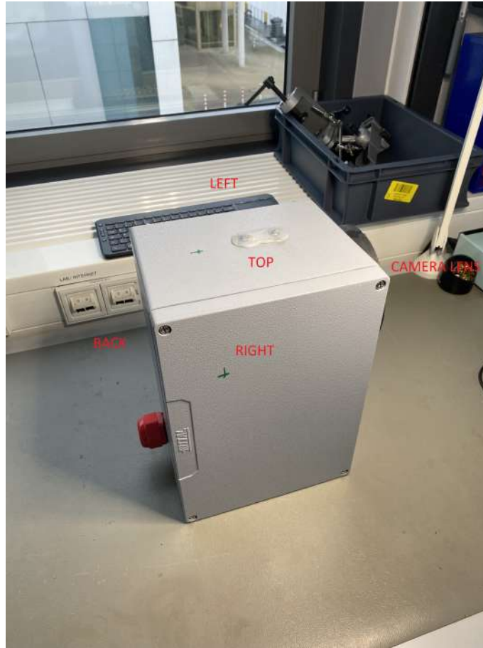
Figure 4.1.: Showcase of the housing, with markings for the possible positions for attaching the smartphone
