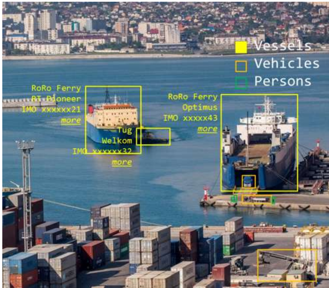
Figure 2.1.: Mock-up example of how ships and other relevant elements at the maritime infrastructure are detected and classified [15].
