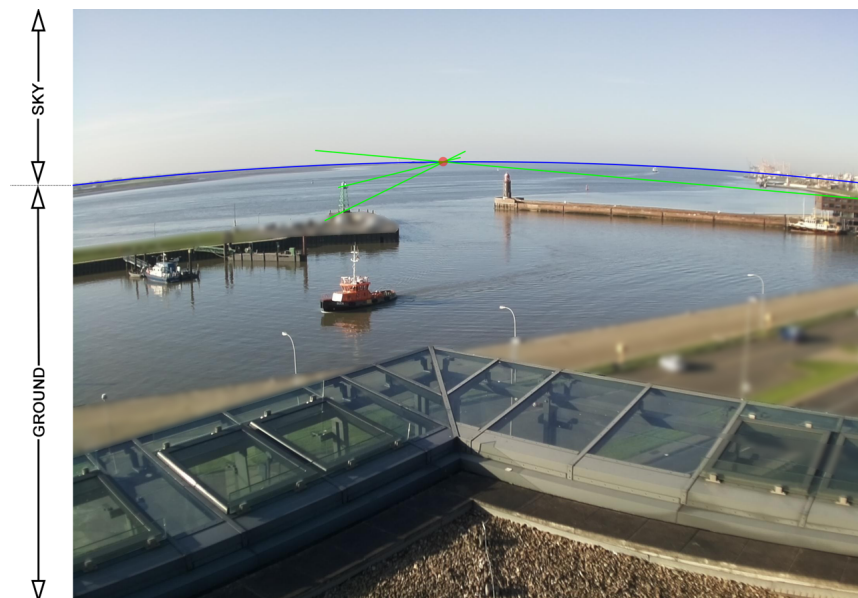
Figure 5.1: Vanishing Point in the ShipSG image vanishing point in red, horizon in blue, reference lines in green
