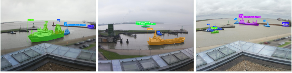
Figure 3.1: Images from ShipSG dataset, showcasing the two camera views and annotated masks and class
