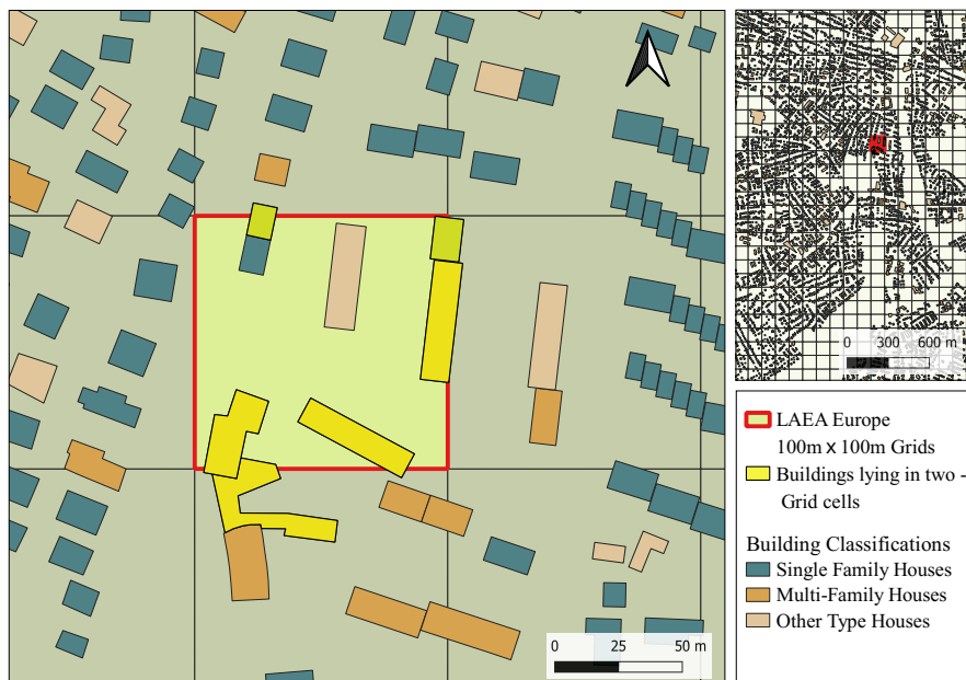
Figure 4-1: Buildings overlapping on multiple grid cells simultaneously
