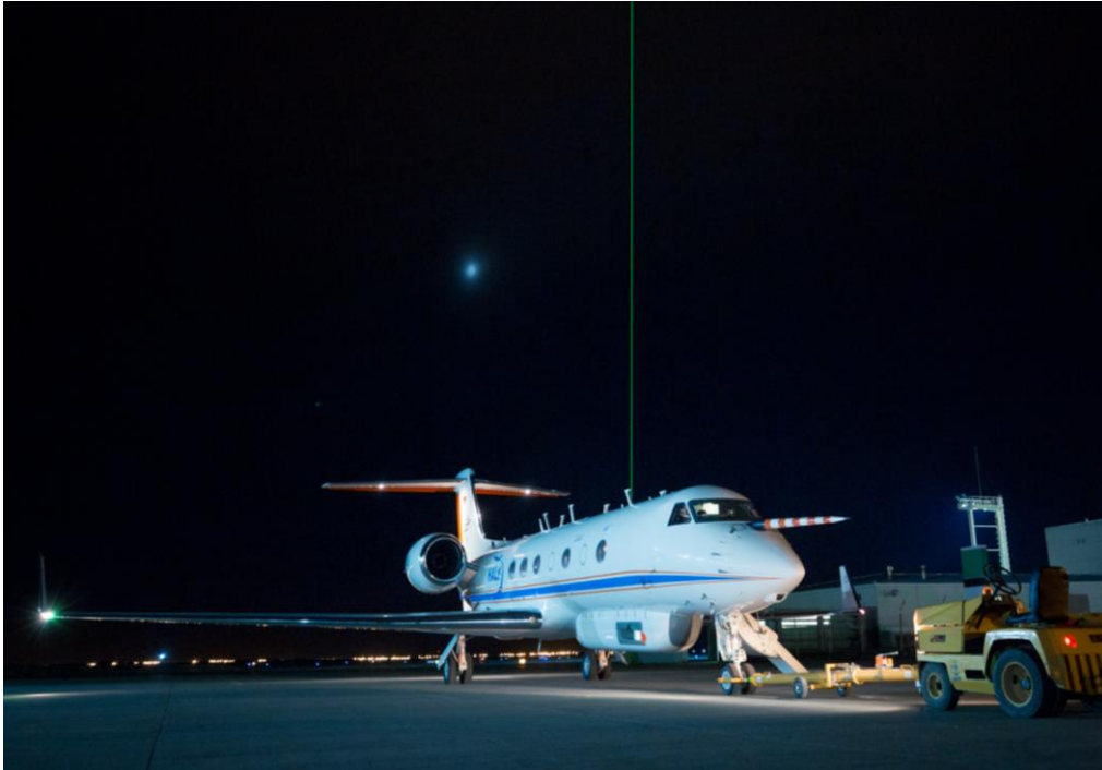
The HALO research aircraft with the laser beam emitted by the ALIMA instrument
