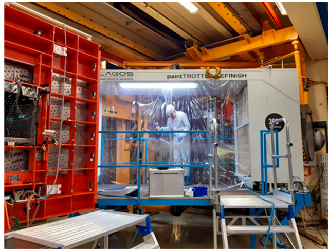
Figure 4. Model coating inside the portable painting booth.
