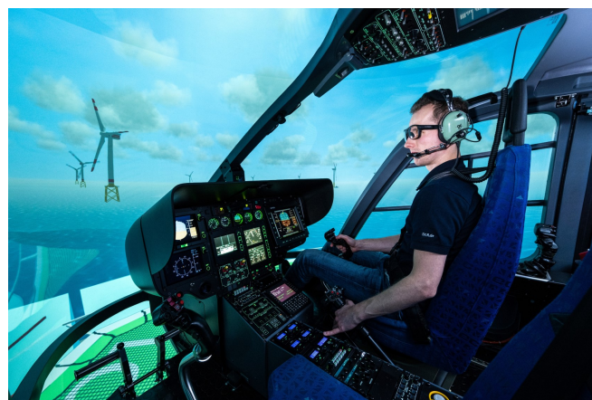
Figure 1. Experimental setup with Eye Tracking in a simulated environment during a final approach in a maritime scenario.
