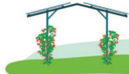
Overhead PV for strawberries cultivation. Source: Baywa r.e.
