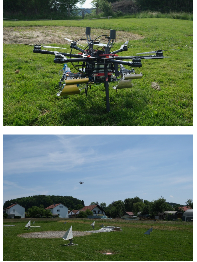
Fig. 2. Pictures of the data acquisition experiment, where a frequency-modulated continuous-wave radar is mounted on a hex-rotor drone (top) and the experiment scene with corner reflectors (bottom), are shown.
