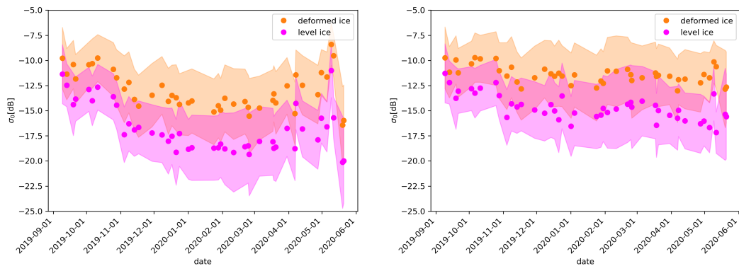
Figure 3.2: Charts showing the mean sigma nought calibrated backscatter for the HH band, for level ice (LI) and deformed ice (DI) from October through May in all labelled scenes. The data is extracted from 52 manually labelled TerraSAR-X scenes. The right hand side shows the chart after correcting for incidence angle dependence using values from Guo et al., 2022 . Note that, because this is only data that was selected manually for training, these values are affected by a selection bias: Only areas are labelled, where the ice type could be determined with high confidence. In reality the contrast between the two classes is most probably smaller.
