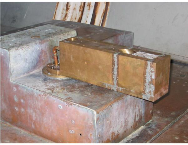
Figure 7: Probe to measure the emission lines under  $90^\circ$  and  $45^\circ$
