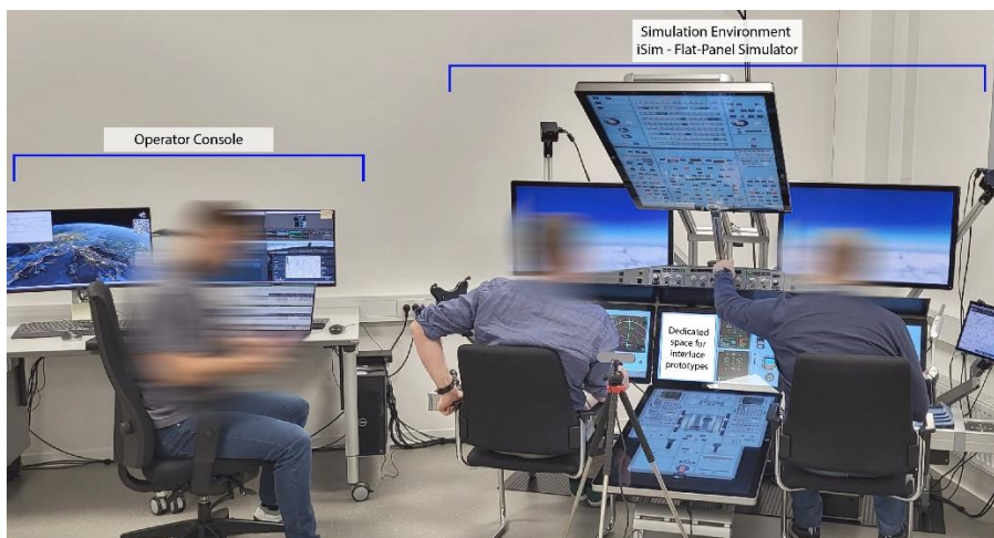
Figure 8. The simulation environment at DLR in Brunswick houses the iSim, a flat-panel simulator that works with touch screens. This allows rapid prototyping without the need to modify hardware.
