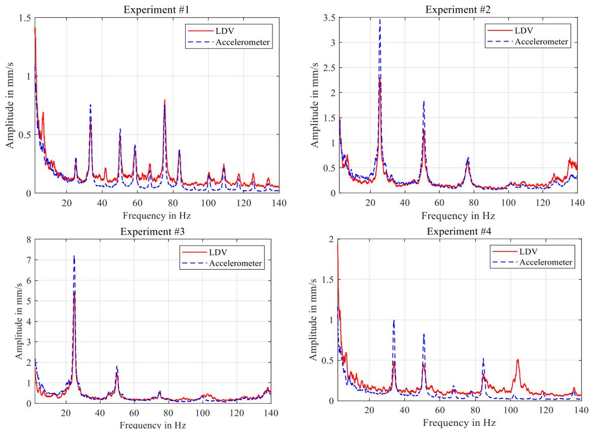
Figure 5. Vibration measurements (resolution bandwidth: 0.9 Hz) with a LDV and an accelerometer acquired from the same target (eccentric shaker in Figure 3).
