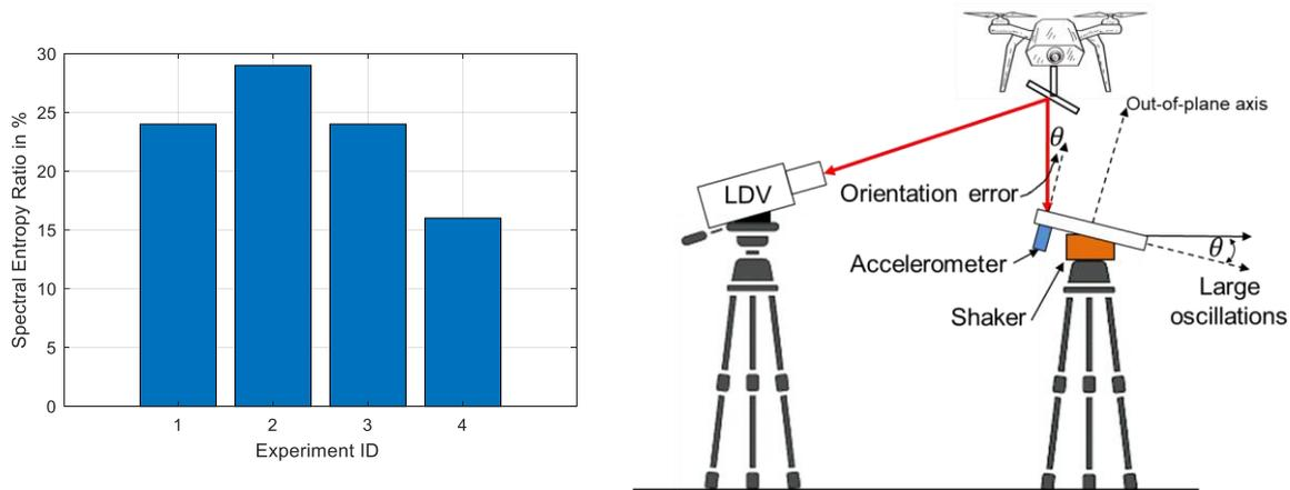
Figure 7. The spectral entropy ratios for all experiments in Figure 5 (left). Example of an unstable measurement position for the shaker table at large amplitudes.
