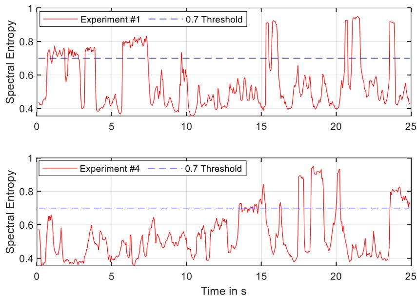
Figure 6. Examples of spectral entropy for LDV measurements for experiments 1 and 4. In experiment 1, about 24% of spectral entropy data (quality index) is above the threshold level of 0.7, while it is only 16% for experiment 4.
