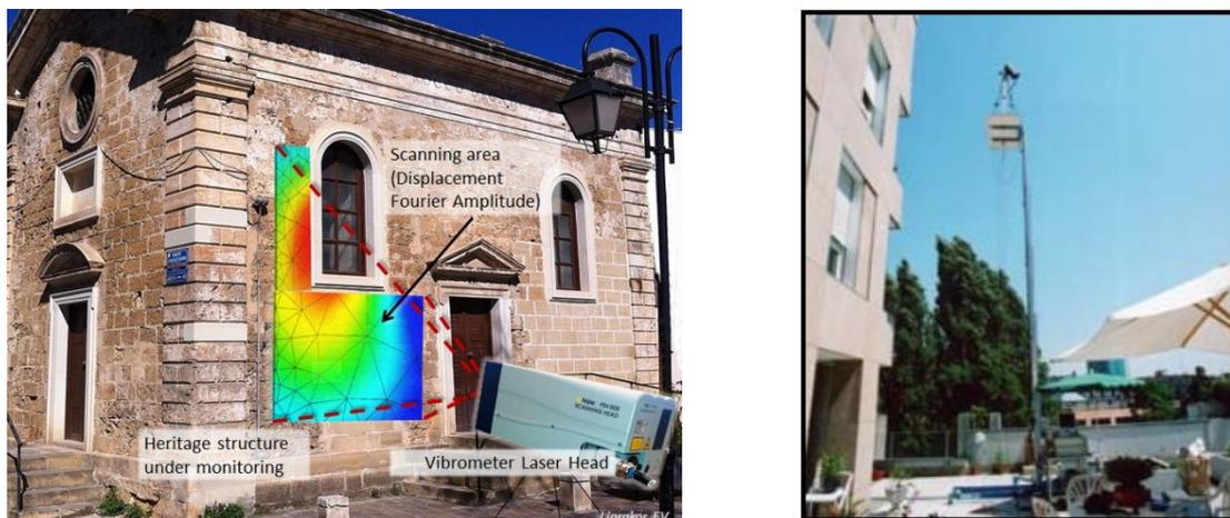
Figure 1. (Right) Laser Doppler vibrometer-based ambient vibration testing for a masonry structure, including a color map for dynamic displacement distribution [11]. A laser Doppler vibrometer is carried by a lifter to monitor a large building [9].
