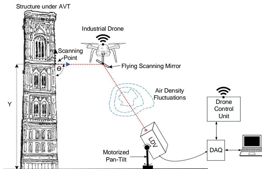
Figure 2. Conceptual design of the Flyable Mirror assembly, including a ground LDV and a reflective mirror installed on a drone. The target structure is under ambient vibration testing.
