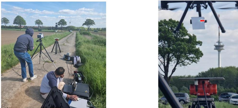
Figure 4. Photographs of the first Flyable Mirror experiment. Drone movement was executed manually. The laser Doppler vibrometer beam on the drone mirror is visible in the right photograph.
