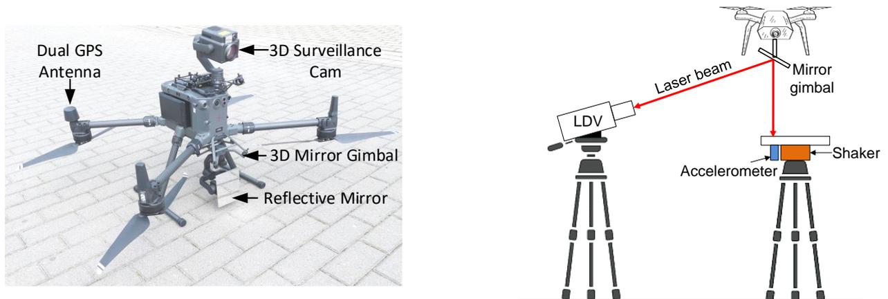
Figure 3. Picture of the drone payloads (left) and schematic of the test setup (right).
