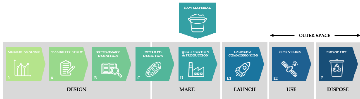
Figure 3.2: Life cycle (in grey) and mission phase (in color) of a space mission (adapted from [30])
