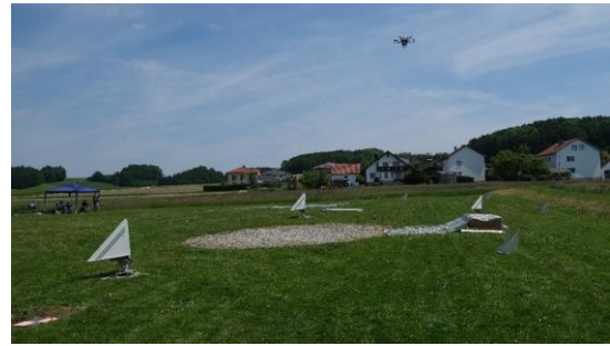
Figure 4 The drone DJI Matrice 600 Pro with the radar system onboard (top) and the test field including the drone, and some corner reflectors (bottom).
