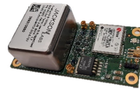
Figure 7 Small lightweight Global Positioning System Disciplined Oscillator (GNSSDO) with a double oven-controlled crystal oscillator (OCXO).
