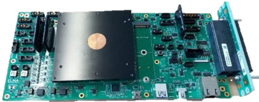
Figure 5 CPU carrier board with COMe Modul, VPX and periphery connection.
