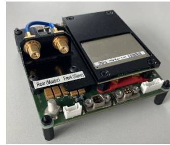
Figure 12 HPINS based on Novatel dual antenna GNSS receiver and Epson IMU
