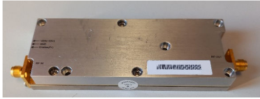
Figure 10 HPA: pulse amplifier with more than 20 W pulsed output power and only 150 g weight
