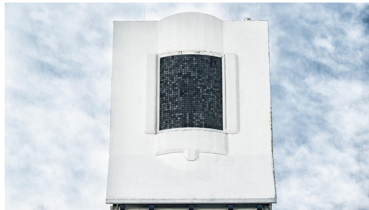
Figure 2.5: The open volumetric receiver, with its 1080 ceramic absorber cups at the solar power plant in Jülich. The air shafts to the sides and the bottom of the receiver surface blow return air to the receiver surface to reduce wind influences (DLR, n.d.).
