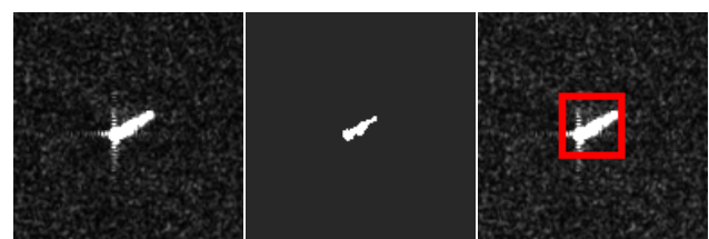
Figure 8 Example of hardware-accelerated CFAR ship detection. Cutout of the pre-processed SAR image (left), binary mask after CFAR kernel (middle) and ship marked by host software after further processing (right).
