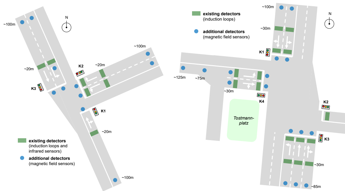
Fig. 2. Setup of detectors at the test intersections in Halle (Saale) (left) and Braunschweig (right).
