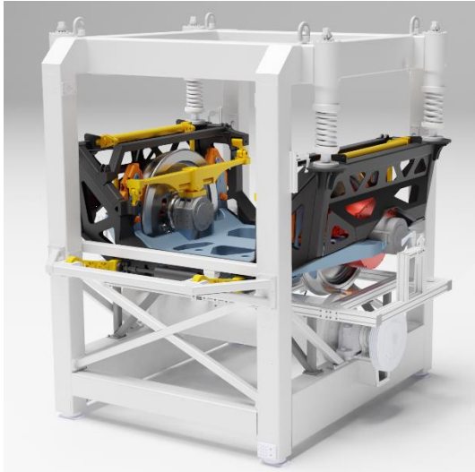
Figure 2: Rendering of the FuN research facility, with the NGT bogie installed in an integration test stand featuring a small roller rig
