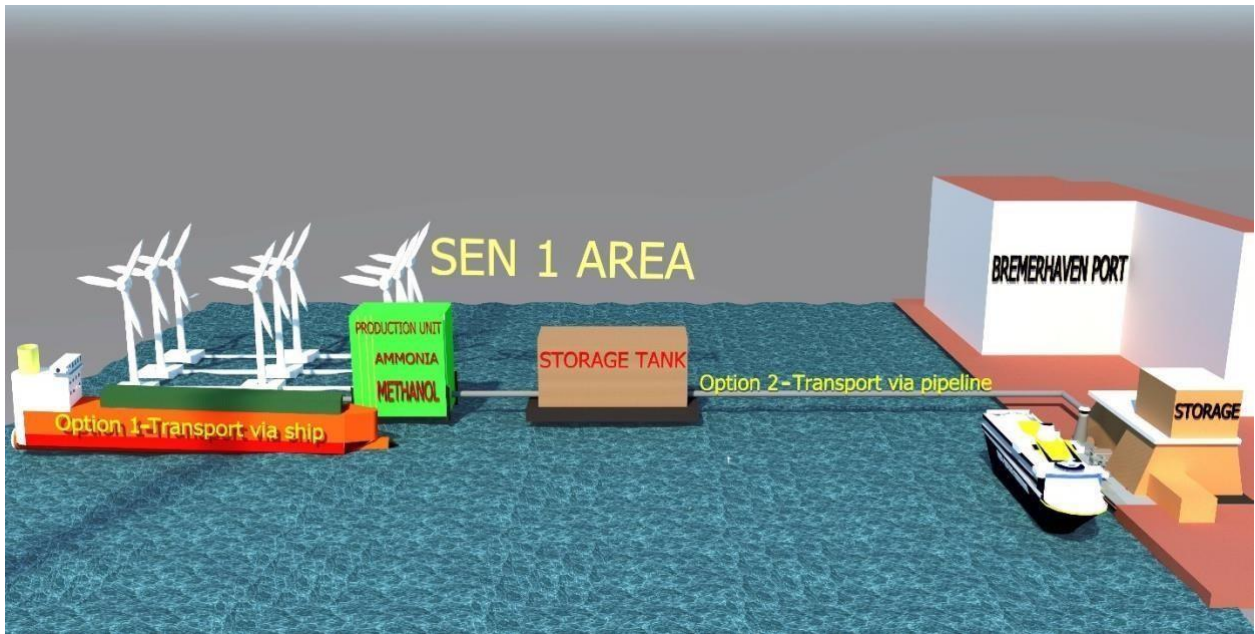
Figure 5- PICTORIAL REPRESENTATION OF TRANSPORT OPTIONS CONSIDERED IN STUDY FROM SEN 1 AREA TO BREMERHAVEN
