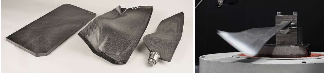
Figure 2 Manufacturing process of the CFRP blades (left) and the shaker test (right)
