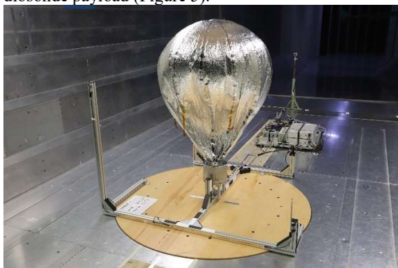
Fig. 3 Wind tunnel test set-up in the German-Dutch (DNW) low speed wind tunnel
