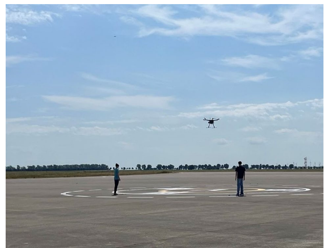
Fig. 1 Demonstration of an aborted landing at a vertiport, due to persons on the ground during our HorizonUAM project. The persons are simulated by puppets
