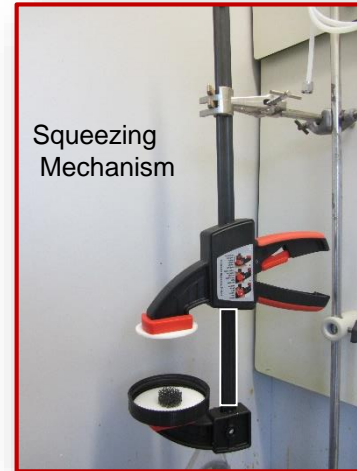
③ Coating & removal of excess slurry
