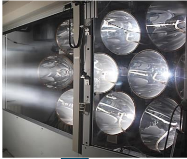
Solar simulator in Cologne (Max. 20 kWth)
