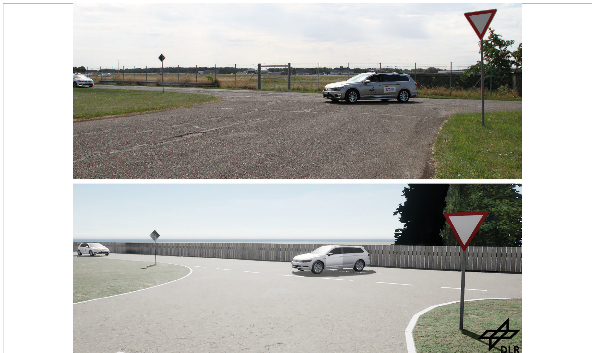
Figure 1: Left turn scenario with driving SAE 4 automation on (top) proving ground and (bottom) within simulation (© Deutsches Zentrum für Luft- und Raumfahrt e. V. (DLR))
