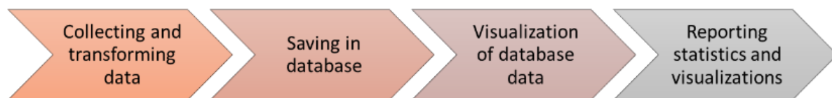
Figure 5: The DFD Monitoring and Reporting process
