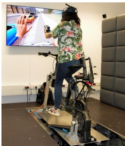
Figure 1. Bicycle simulator at the MoSAIC-VRU-Lab
