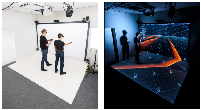
Figure 4: The Virtual Reality lab at the German Aerospace Center in Brunswick, Germany is used regularly to evaluate the framework described in this paper. The lab uses four stereo projectors (three for the back projection and one for the floor projection). Each projector is connected to a separate workstation. Images courtesy of German Aerospace Center, DLR (CC-BY).
